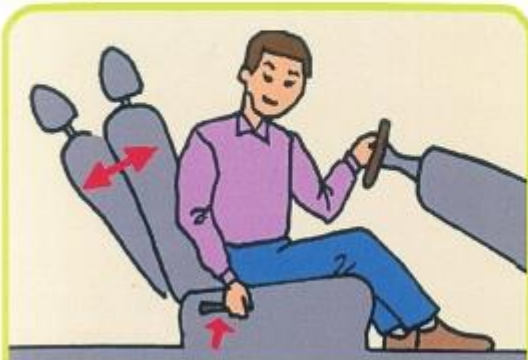
Left hand holding steering wheel, lift adjustment lever on the right of the seat with right hand. Lean seat forward and backward using body.
