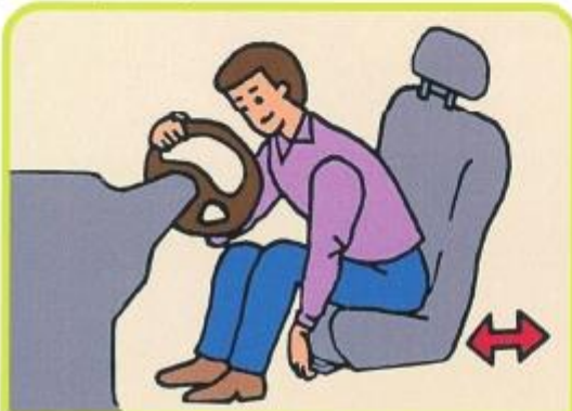
Right hand hold steering wheel. Lift adjustment lever under left side of the seat with left hand and slide seat forward/backward.
